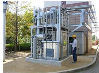
Test equipment to capture CO<sub>2</sub>
