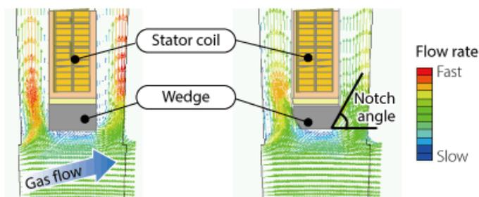
Reducing windage loss by improving the cross-sectional structure of stator coils
