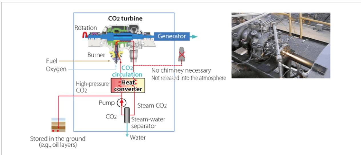
Actual-pressure combustion test (Toshiba succeeded in achieving combustion at the target atmospheric pressure of about 300,000 hectopascals.)
