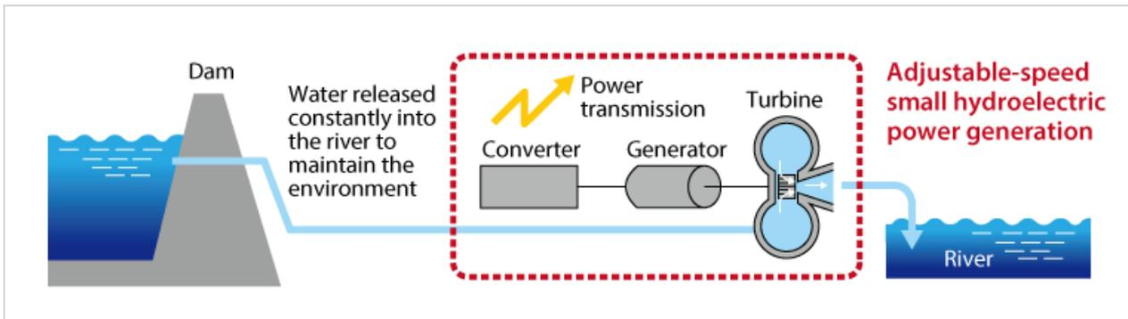
Structure of an adjustable-speed small hydroelectric power generation system
