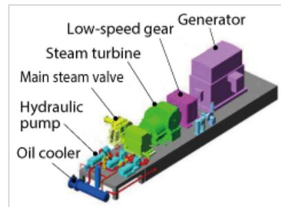
Compact geothermal turbine generator
