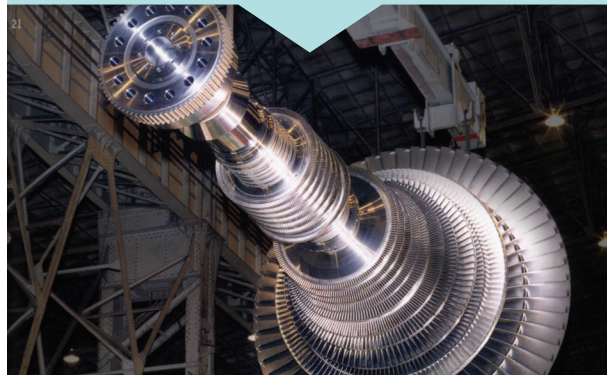
TOSHIBA'S STEAM TURBINE
